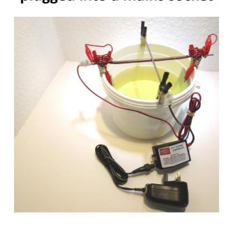
A crocodile lead is now connected to the non sleeved item bar and the other end is connected to the item being plated. The lead is tied to the item bar so that the item being plated is suspended in the plating solution
