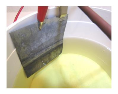
At the end of plating the item is lifted from the plating tank using the lead so it is not handled before rinsing and the passivation stage
