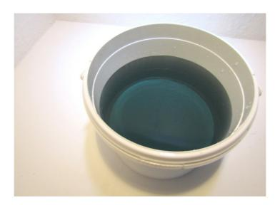
The plated and rinsed item is simply lowered into the blue passivate solution for 15 to 45 seconds
