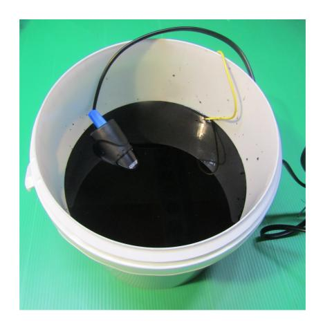
The plated item is then simply lowered into the pre heated yellow passivate solution for between 90 and 120 seconds depending on the depth of colour desired. The yellow passivate solution should be agitated for the duration of the dip time by either, moving the part gently around in the solution, stirring the solution with a non metallic stick, or using an air supply agitator. The item should then be then thoroughly rinsed.
