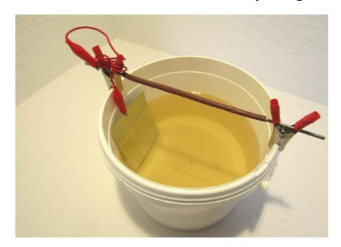
The anode lead is tied around the anode rod so that the submerged area of anode is roughly equivalent to the area of the item being plated
