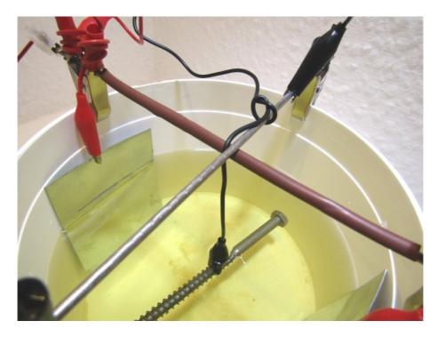
AVOID hanging the parts on wire, this is not a suitable method of providing an electrical supply to the parts.
