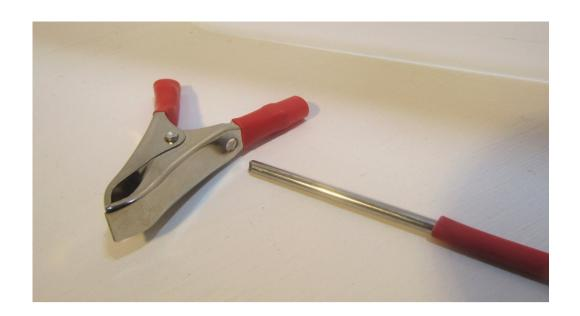
THE RED SLEEVED ANODE ROD IS PUSHED THROUGH BOTH HOLES IN A RED SUPPORT CLIP
