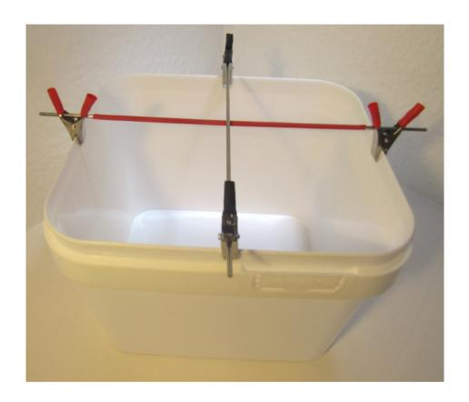
REPEAT THE SAME PROCEDURE FOR THE NON SLEEVED ROD USING THE 2 BLACK SUPPORT CLIPS AND CLIP THIS ROD ONTO THE SIDES OF THE TANK SO THAT THE ROD IS AT 90 DEGREES TO THE RED SLEEVED ROD
