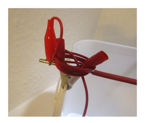
A CROCODILE CLIP LEAD IS NOW INSTALLED ONTO THE RED SLEEVED ROD SO THAT AN ELECTRICAL CONNECTION IS MADE BETWEEN THE RED SLEEVED ROD AND THE ANODE, WHICH WILL BE SUSPENDED IN THE PLATING SOLUTION. THE LENGTH OF LEAD ON THE INSIDE OF THE TANK THAT WILL CLIP ONTO THE ANODE CAN BE ADJUSTED DEPENDING ON THE VOLUME OF PLATING SOLUTION AND THE SURFACE AREA OF ITEMS TO BE PLATED ENSURING THAT THE CROCODILE CLIP DOES NOT CONTACT THE PLATING SOLUTION
