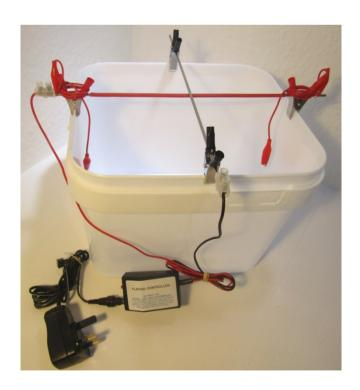
THE POWER SUPPLY IS NOW PLUGGED INTO THE CONTROL UNIT AND IT SHOULD BE CONNECTED TO THE MAINS SUPPLY BEFORE PLATING BEGINS
