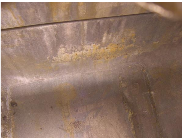
Rusty Old Tank Before Using POR15 Tank Sealer
