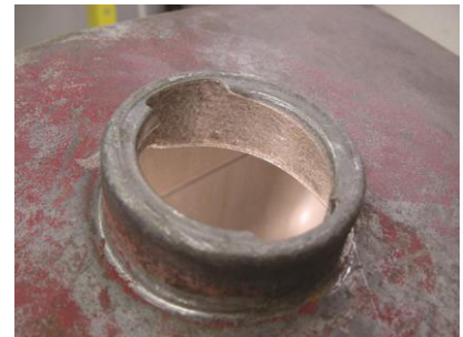
POR15 Tank Sealer - After
